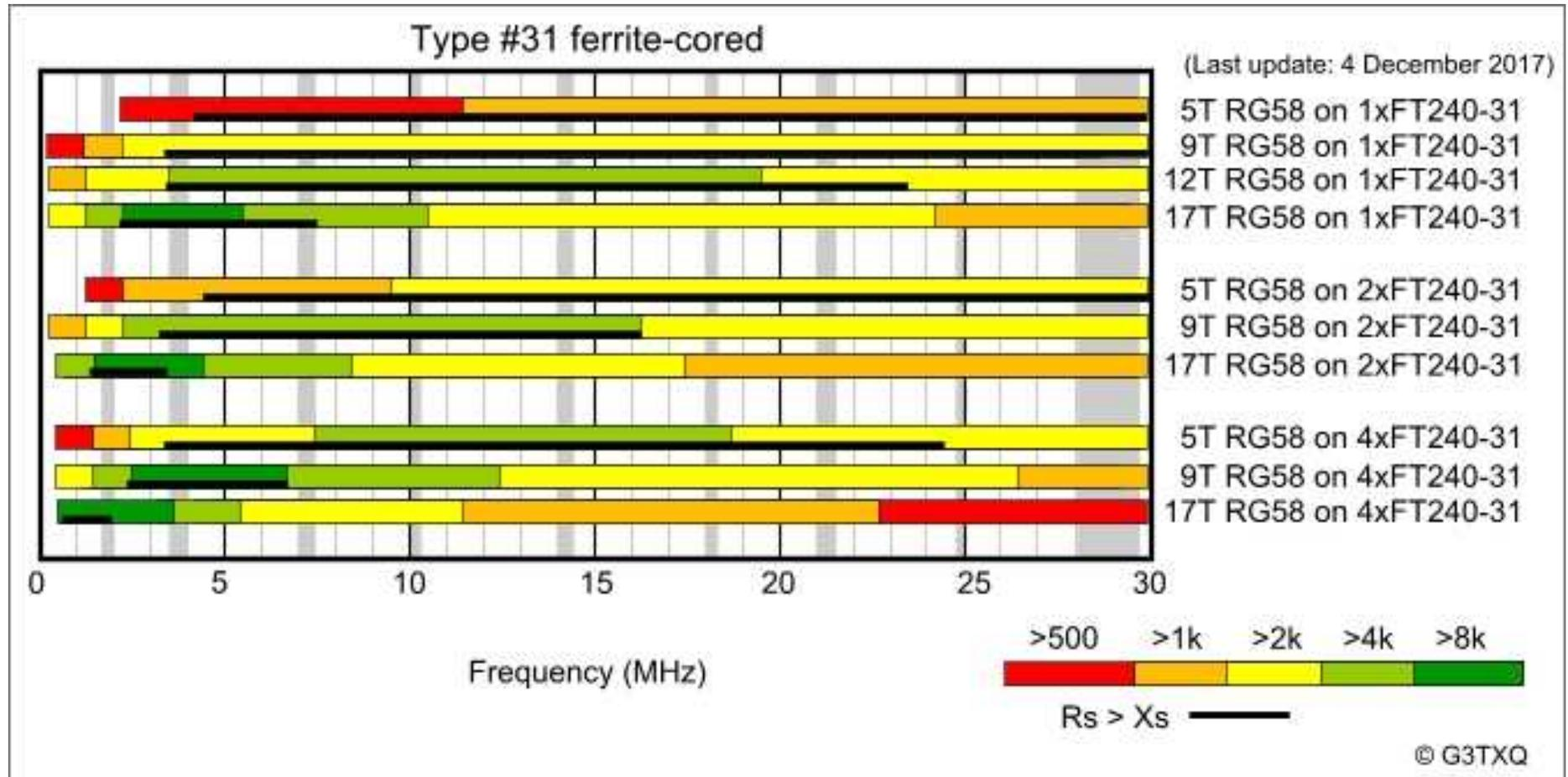
Measurements on combinations of 5 turns, 9 turns, 12 turns and 17 turns on single, 2-stacked and 4-stacked
